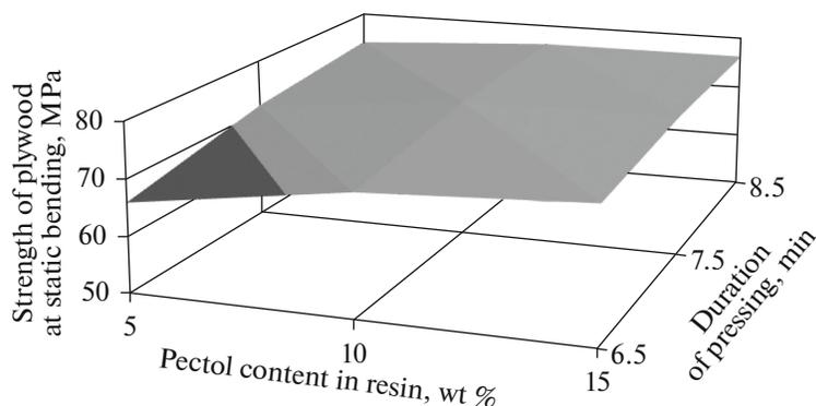
**Fig. 1.** The dependence of the strength of plywood at static bending on the content of pectol in SFZh-3013 resin and the duration of pressing.
