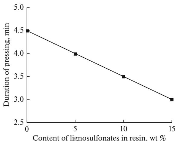
**Fig. 4.** The dependence of the duration of pressing of plywood on the content of lignosulfonates in KF-MT-15 resin.
