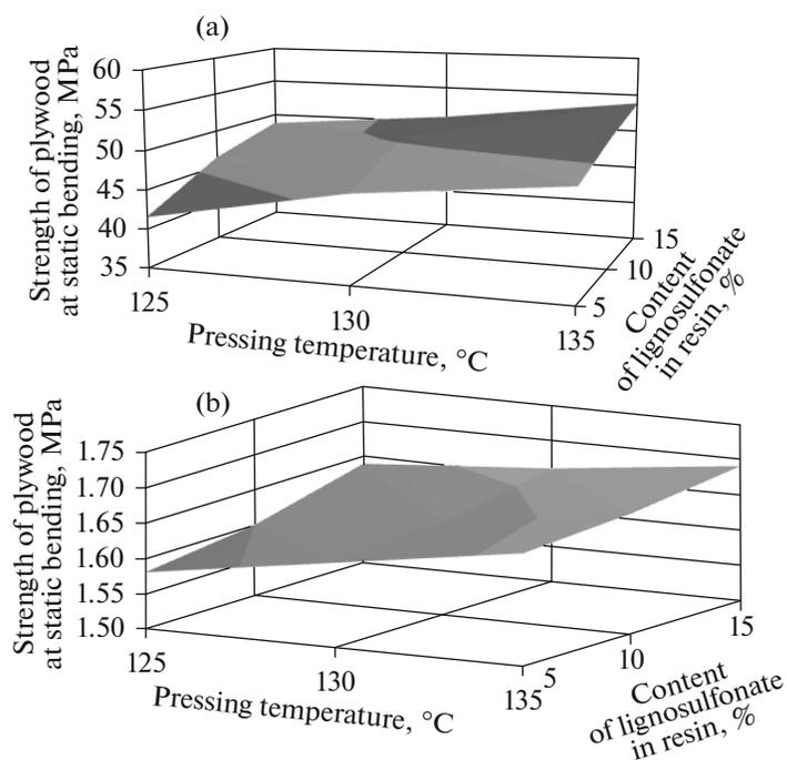
Fig. 5. The dependence of the strength of plywood at (a) bending and (b) shearing on the content of lignosulfonates in KF-MT-15 resin and the temperature of pressing.
