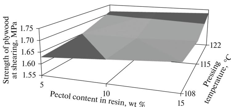
**Fig. 2.** The dependence of the strength of plywood at shearing along the fibers on the content of pectol in the SFZh-3013 resin and the pressing temperature.
