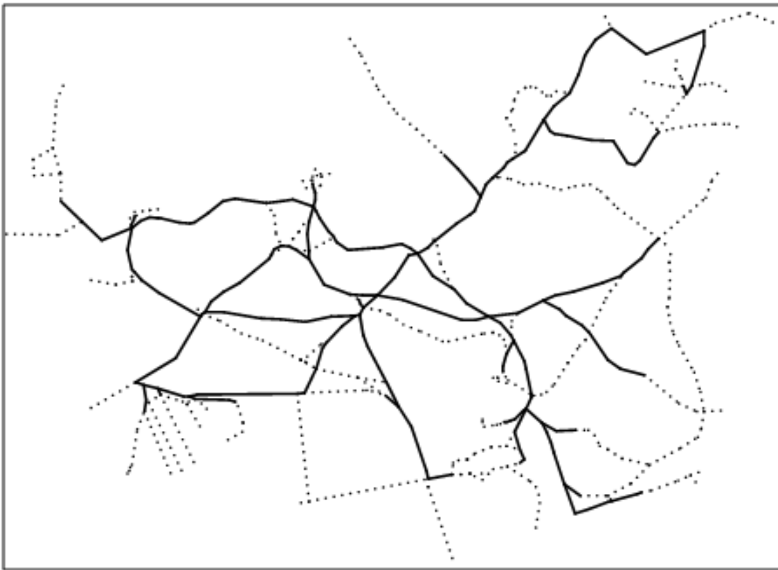
Fig. 2. Angular segment model of the Osinovaya Roscha forest park study area. Segments where LN(\text{choice}) \geq \text{Avg}(LN\text{choice}) are represented with solid lines, segments where LN(\text{choice}) < \text{Avg}(LN\text{choice}) are represented with dashed lines.
