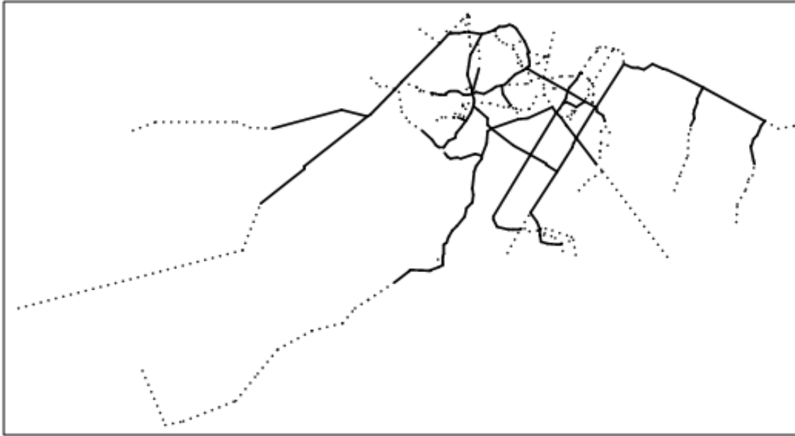
Fig. 1. Angular segment model of the Pesotchny forest park study area. Segments where LN(\text{choice}) \geq \text{Avg}(LN\text{choice}) are represented with solid lines, segments where LN(\text{choice}) < \text{Avg}(LN\text{choice}) are represented with dashed lines.
