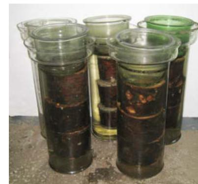
20-sm bolts of Siberian fir submerged in buckets with cold water for 1 to 4 weeks (3 bolts for each treatment).
